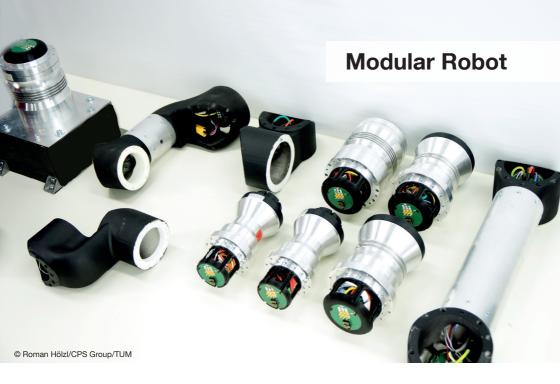
In this demo, visitors can experience the first truly modular industrial robot arm. The key technologies are fully modular and self-contained hardware modules and the self-programming of the robots' control and collision check. After reading kinematic and dynamic data, which is saved on every robot module, a centralized controller is programmed on-the-fly, which enables instant usage of newly assembled or reassembled modular robots.
