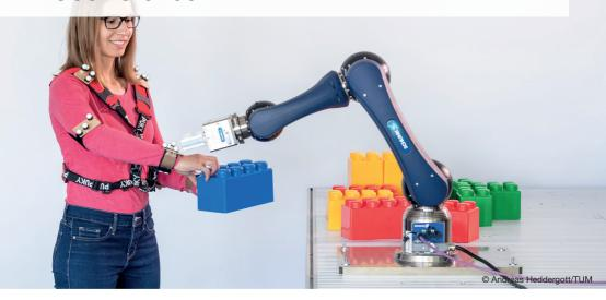
In this demo, visitors can experience what working is like in close proximity to an industrial robot arm that behaves reliably safe in presence of humans. The key technology are computationally efficient methods that formally verify the safe behavior of robotic systems at runtime. By using human pose recognition (from an installed motion capture system) and the prediction of their reachable sets, we achieve higher productivity at work while retaining the same safety requirements for humans.
